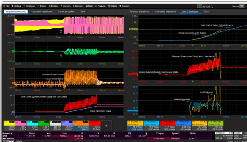
Measured losses are compared to drive control system estimated losses and further calculations are made to separate measured losses into core (iron) and load (copper) losses.
