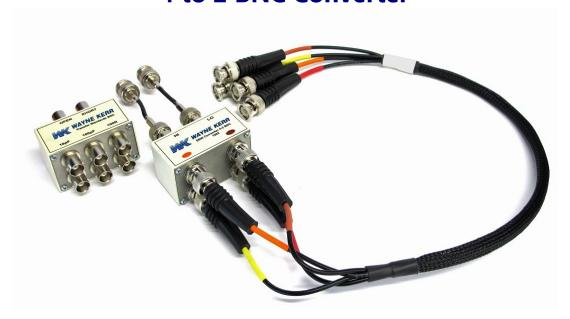
The 1J1001 4 to 1 BNC Converter is used to connect a Wayne Kerr 6500 analyzer to the Device Under Test which is terminated in two BNC connectors.
