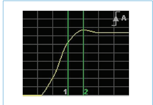
Figure 3b. Waveform analysis with time 10 ns/div time base and 1 sample per division.
